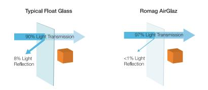
In addition, the carefully tailored anti-reflective coating utilised in AirGlaz has been specially designed so that any reflection caught in the 1% factor appears in a dark blue rather than the pink area of the spectrum, helping to remove unwanted glare and prevent distortion.
